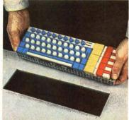
KB allows bench assembly. Assemble a complete keyboard matrix at the bench where the job is easier, faster. Even the wiring is done before the matrix is set into the console.
